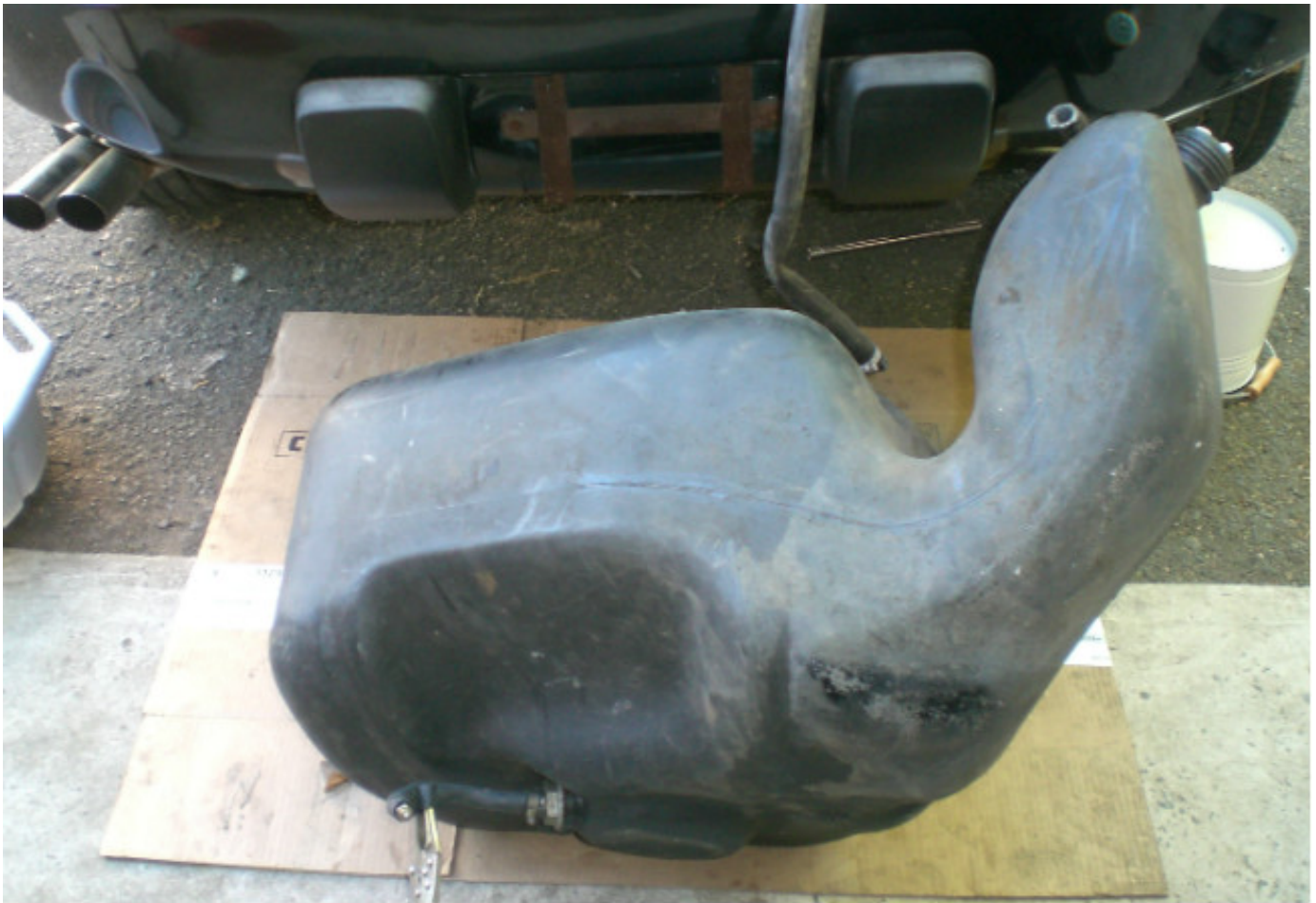
The "ostrich" as it's known in Porsche tech parlance. Cracked fuel tanks seem to plague lots of these early 928s, so be aware of this should you be in the market for one.
